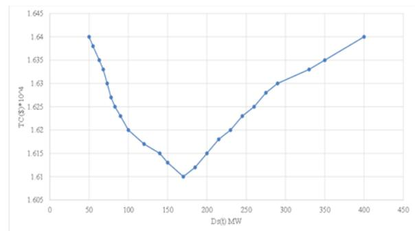
**Fig. 3. the overall cost based on the function of the spinning reserve for the 1430MW load level**
