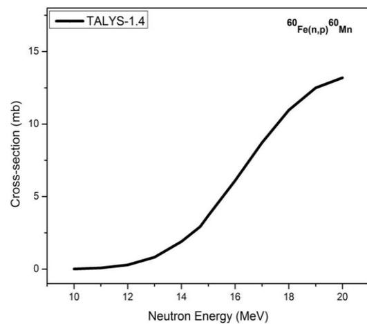
**Fig.4. Excitation function of the  $^{60}\text{Fe}(n,p)^{60}\text{Mn}$  reaction.**
