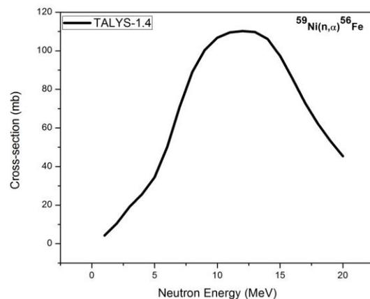
**Fig.12.** Excitation function of the  $^{59}\text{Ni}(n,\alpha)^{56}\text{Fe}$  reaction.
