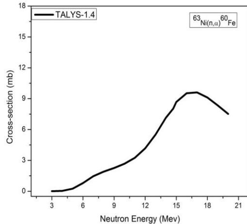
**Fig.13. Excitation function of the  $^{63}\text{Ni}(n,\alpha)^{60}\text{Fe}$  reaction.**
