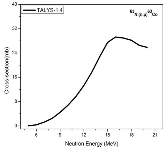
**Fig.7. Excitation function of the  $^{63}\text{Ni}(n,p)^{63}\text{Co}$  reaction.**
