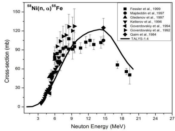
**Fig. 11.** Excitation function of the  $^{58}\text{Ni}(n,\alpha)^{55}\text{Fe}$  reaction.
