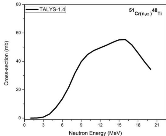
**Fig. 8. Excitation function of the  $^{51}\text{Cr}(n,\alpha)^{48}\text{Ti}$  reaction.**
