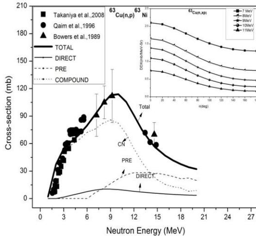
**Fig. 2. Excitation function of the  $^{63}\text{Cu}(n,p)^{63}\text{Ni}$  reaction along with double differential cross-sections (DDX) with angle of emission for 7,8,9,10 and 11 MeV proton particles emitted through  $^{63}\text{Cu}(n,xp)$  reaction at 14MeV neutrons.**
