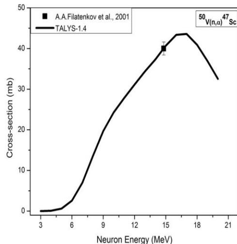
**Fig. 14. Excitation function of the  $^{50}\text{V}(n,\alpha)^{47}\text{Sc}$  reaction.**
