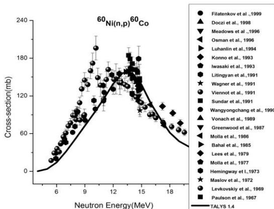
**Fig.6. Excitation function of the  $^{60}\text{Ni}(n,p)^{60}\text{Co}$  reaction.**
