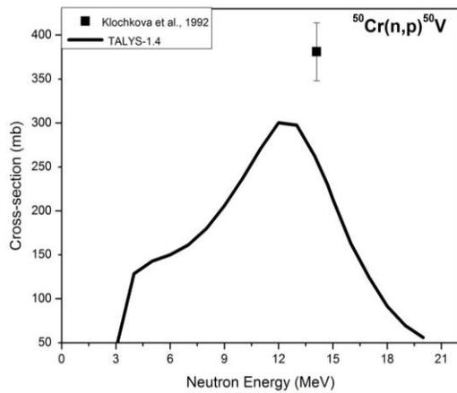
**Fig. 1. Excitation function of the  $^{50}\text{Cr}(n,p)^{50}\text{V}$  reaction.**
