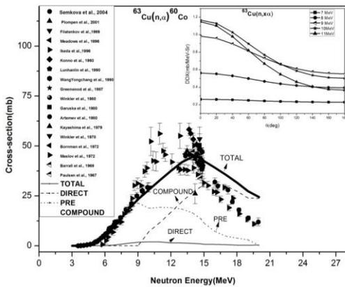
**Fig. 9.** Excitation function of the  $^{63}\text{Cu}(n,\alpha)^{60}\text{Co}$  reaction along with double differential cross-sections (DDX) with angle of emission for 7,8,9,10 and 11 MeV alpha particles emitted through  $^{63}\text{Cu}(n,\alpha)$  reaction at 14 MeV neutrons.
