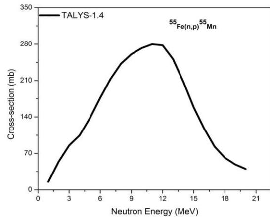
**Fig.3. Excitation function of the  $^{55}\text{Fe}(n,p)^{55}\text{Mn}$  reaction.**
