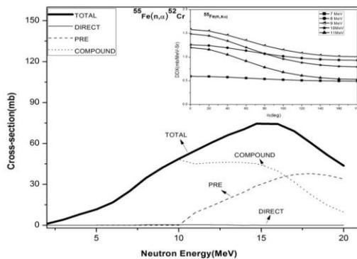
**Fig. 10.** Excitation function of the  $^{55}\text{Fe}(n,\alpha)^{52}\text{Cr}$  reaction along with double differential cross-sections (DDX) with angle of emission for 7,8,9,10 and 11 MeV alpha particles emitted through  $^{55}\text{Fe}(n,\alpha)$  reaction at 14 MeV neutrons.
