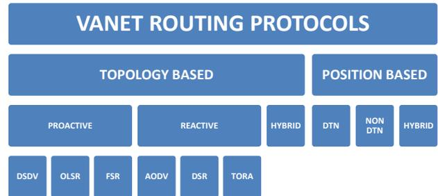
FIG. 3 VANET ROUTING PROTOCOLS
