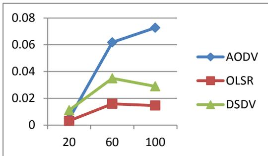
FIG. 5 PERFORMANCE GRAPH OF DELAY FOR 20, 60 AND 100 VEHICLES
