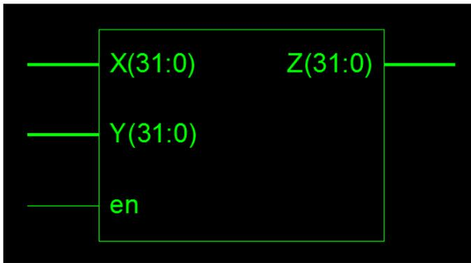
**Fig. 2 Block structure of 32- bit booth multiplier**
